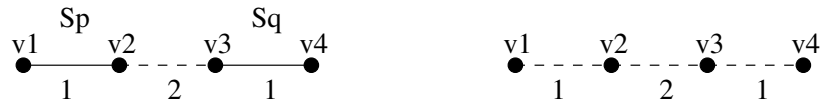
Figure 3: An example collision when vertices with positive gains migrated simultaneously result in an increase in cost.
